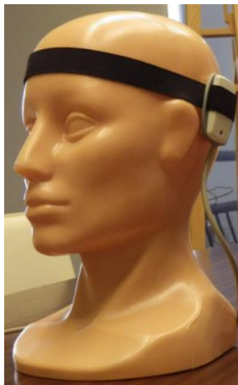
Figure 1: Mounting of the Accelerometer module on the user head.
